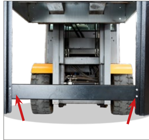
7 - After carefully tightening each bolt, proceed with mounting the 4 support bars using the bolts and nuts.
